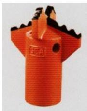
Normally, this is the first choice if there are no hard rock bands. A very cost effective bit giving high installation rates. This bit cuts with a shear action to slice and mix the material being cut. Unlike other bits, the flushing holes are positioned behind the cutting blade to move material quickly away from the drill head. The hardened blades enable the bit to cut through tough Clays, Sand and weak Rock bands.
