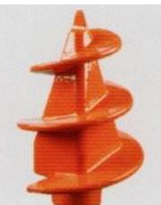
This displacement bit can help prevent the expensive removal of waste material from projects such as highway development, tunnels and toxic sites. The square design reduces skin friction to enable faster installation (up to 8 metres per minute in soft ground), saving time and money. As no flushing is required, further savings are made on reduced grout quantities.
