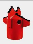
For clays and soft or medium soils, the strong SEA- Cross-Cut drill bit is made from tough cast steel and reaches the desired pile depth with ease. Grout / flushing holes situated behind the cutting blade deliver optimum flow to create a well-formed high load bearing pile. The drill bit is sacrificial and will remain at the bottom of the pile acting as a strong anchor for the tubular steel core.
