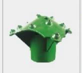
For hard rock, irregular boulders and landfill conditions, the SEA- Domed Button drill bit will provide unrivalled performance. This unique bit is made from a tough steel casting and incorporates high-grade tungsten buttons inset into conica pillars to maximise rock break-up and dispersal. Like the Cross-Cut, the Domed-Button bit is sacrificial and will provide a solid anchor at the bottom of the pile.
